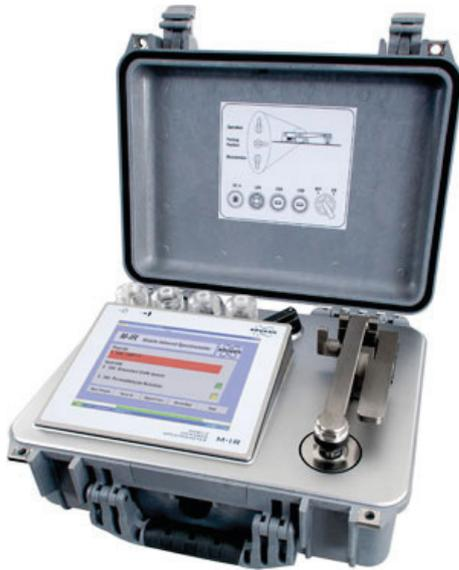
Abb. 1: Mobiles Infrarotspektrometer ([www.photonics.com](http://www.photonics.com))
