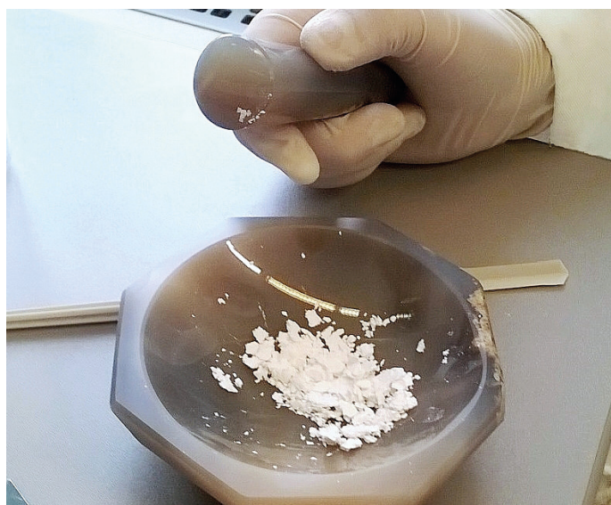
Fig. 1 Crushing the blank filter with mortar and pestle (own photo)
