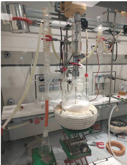
Abb. 1: Syntheseapparatur – Polyolsynthese.
